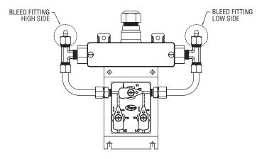
Figure 2: Bleed Fitting Connections
