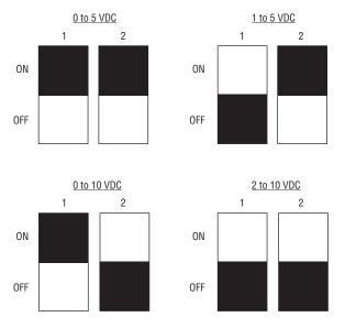
Figure 5: Voltage Output Dip Switch Selection
