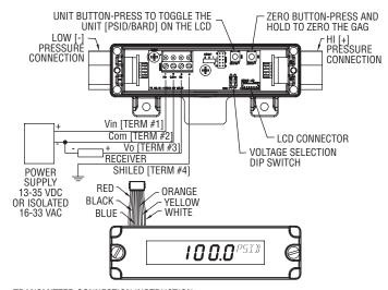
TRANSMITTER CONNECTION INSTRUCTION: - TURN OFF POWER SUPPLY.
