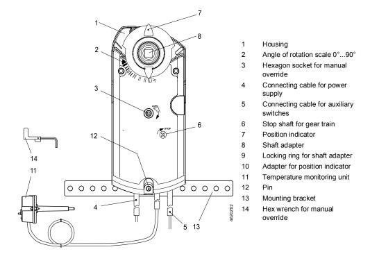
Arrangement for shaft adapters
