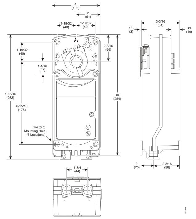
M9220-xxx-3 Electric Spring-Return Actuator Dimensions, in. (mm)
