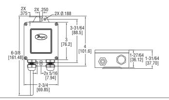
The **SERIES O-4** Outside Air Temperature Sensors are great for monitoring ambient air temperatures in outdoor applications. The temperature sensors are mounted in a NEMA 4X enclosure with integral mounting tabs.
