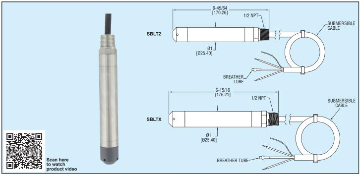
SBLT2 and SBLTX Submersible Level Transmitters are manufactured for years of trouble free service in the harshest applications. Both measure the height of liquid above the position in the tank referenced to atmospheric pressure. The transmitters consist of a piezoresistive sensing element, encased in a 316 SS housing. Bullet nose design protects the diaphragm from damage.
