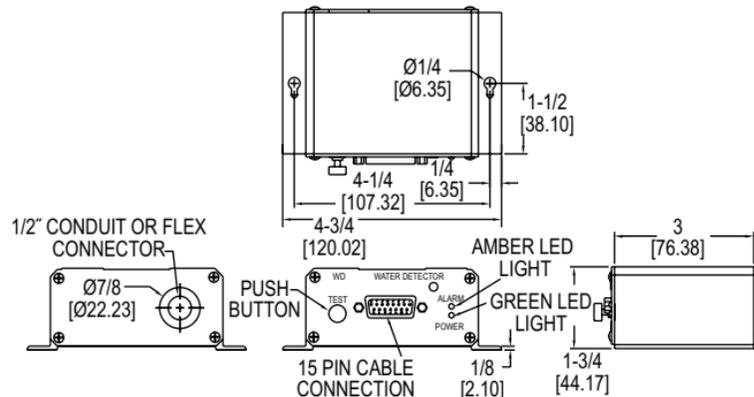
The **SERIES WD** Water Detectors and Sensor Tapes is designed for dependable detection of water presence even of low conductive liquids. The water sensing tape attaches to module and if any liquid comes in contact with the tape the resistance is changed and the alarm will be triggered. The sensing tape is 1" wide and can be bought in lengths of 5, 10, 15 and 25' and is powered by 24 VAC or 24 to 30 VDC.
