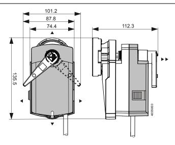
► = >100 mm ► = >200 mm Min. clearance from ceiling or wall for mounting, connection, operation, maintenance, etc.
